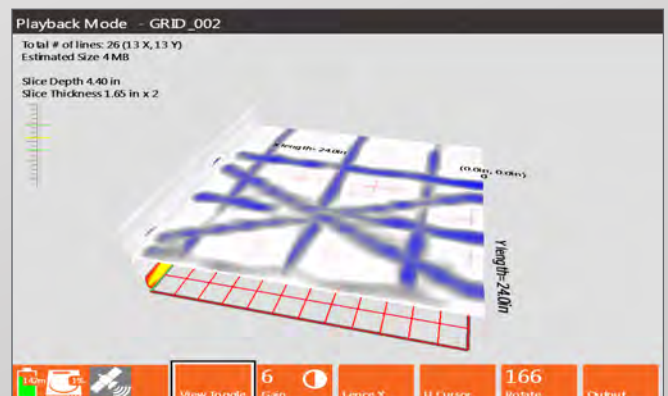
Screen capture of 3D data image. Data illustrates a rebar mat with post tension cables in an "X" pattern.
